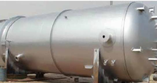
Tank insulation in tank and silo insulations, we insulate with aluminum coating, stainless sheet coating, embossed sheet coating, galvanized coating materials on rock wool and glass wool.
